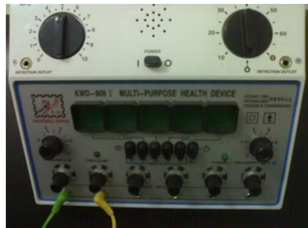
Fig. 2 The KWD-808 electro-stimulator equipped with built-in timer can produce five different waveforms
